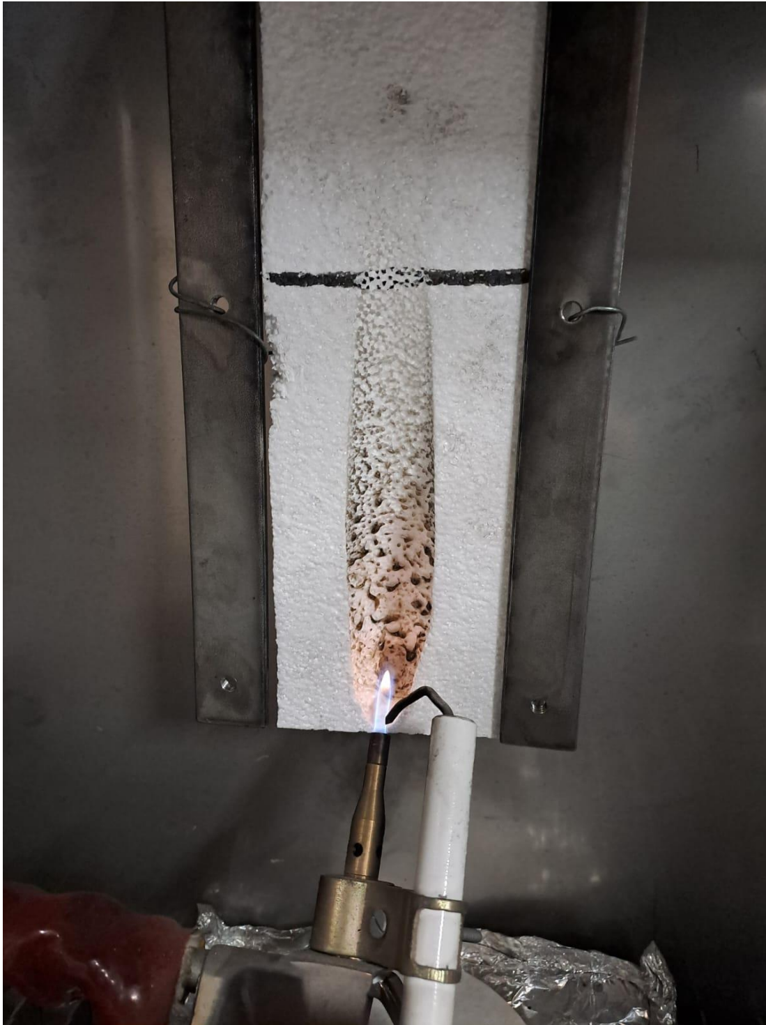
Figure 13: End of ignitability test
