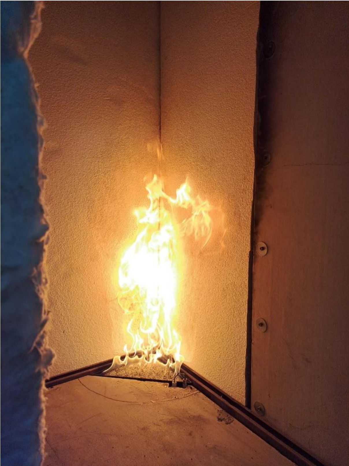
Figure 6: Start of Single Burning Item test
