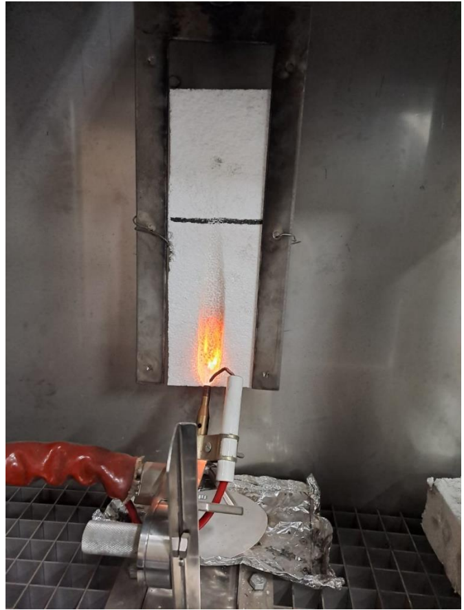
Figure 8: Ignitability test in progress
