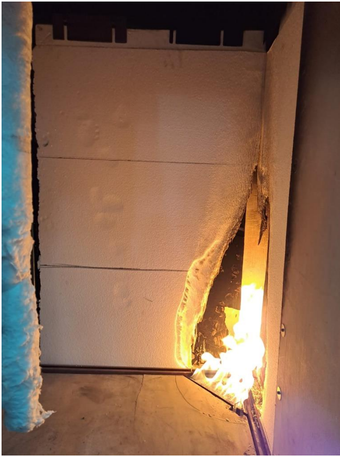
Figure 4: First run Single Burning Item Test in progress
