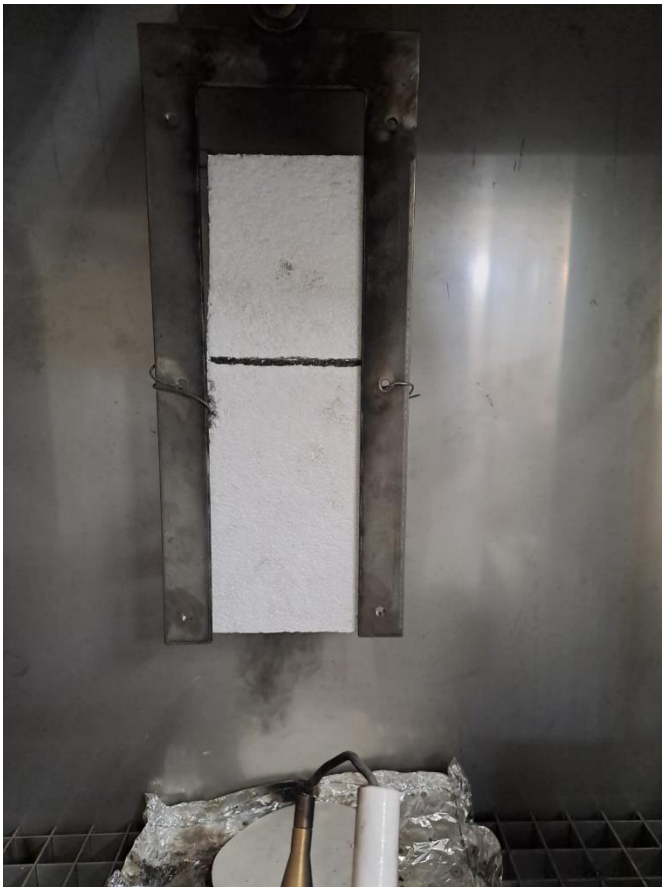
Figure 7: Ignitability test sample
